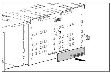
Figure 2-17. Removing the Simplex Enabler Board
